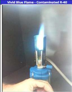
Flame may start as green colour, but as more flow of refrigerant passes through, then it dramatically turns to an electric blue colour and onwards to vivid blue/purple. This is most likely R-40 mixed with other CFC refrigerants and R-134a. This is what caused the explosions when unit was powered up and reacted with moisture at 473°C.
