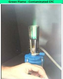
Flame can easily be seen to change to a green tinge as the Chlorine in the refrigerant (CFC) reacts with the copper reaction plate. Most likely cause is a mixture of R-22 and/or R-142b which is cheaper than R-134a.
