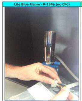
Flame is almost invisible but has a lite blue central core where the gas flame reacts with the copper reaction plate. As R-134a passes through the testing hose there will be a slight waving of the flame as it burns the refrigerant excess flow will cause roange flame (lack of oxygen) and eventually flame extenguished.
