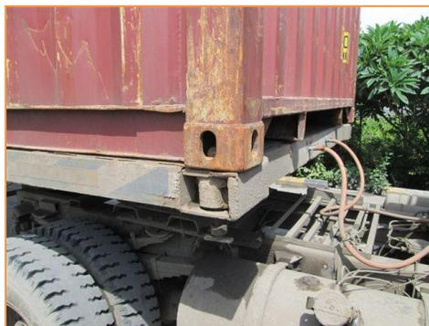
**Checking tractor trailers for stuck/improper Twist Locks inside the Terminal area**
